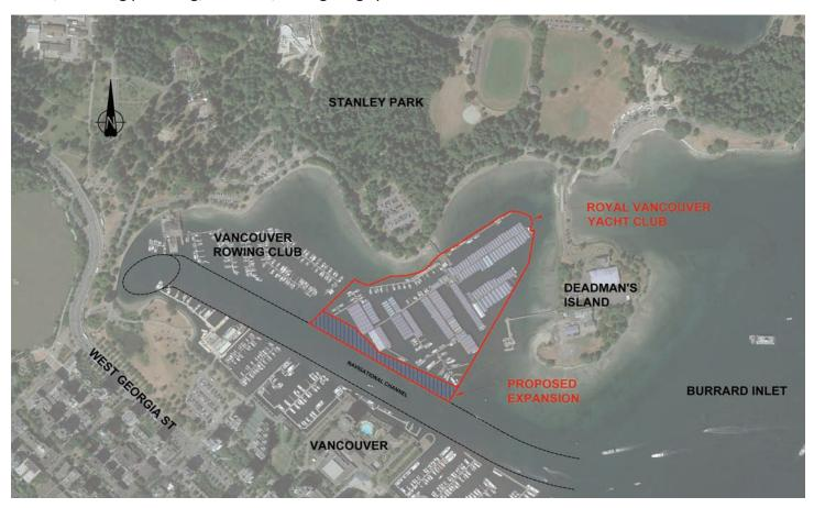
**Phase 1** - Construction of K float, along with the outer edge of the new water lot adjacent to the channel. Works will be undertaken in proximity to, but not within, the navigational channel, and may have some minor effects on marine stakeholders.
